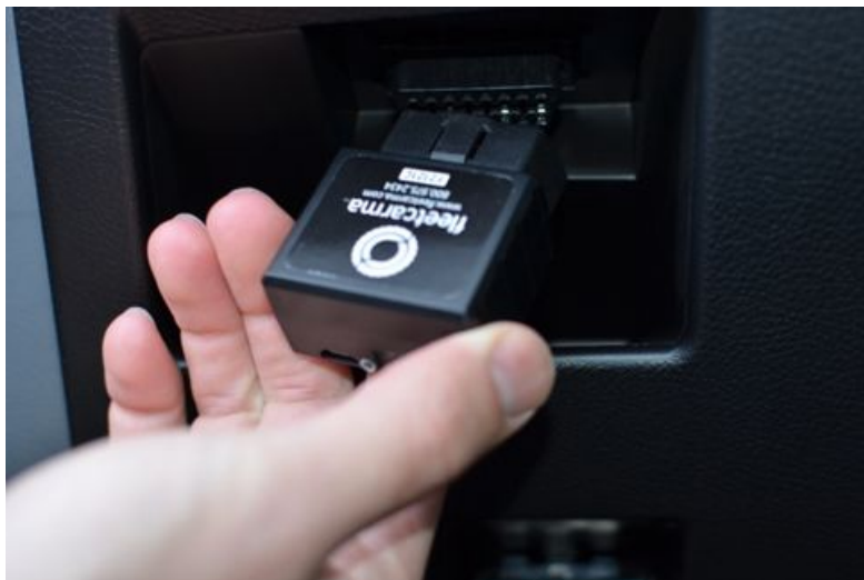
Figure 1: Installation of a FleetCarma C2 Device into a Vehicle's Diagnostics Port
